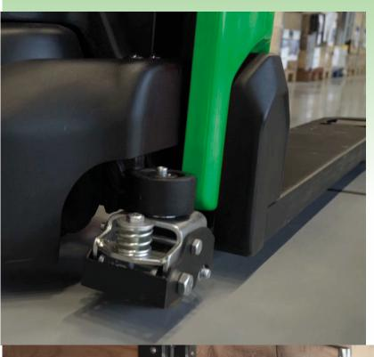
Easy long-side pallet handling. Twin fork wheels as standard, for reduced pressure on floors and easier and silent travel over uneven surfaces.
