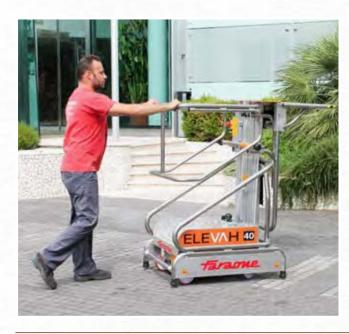
PUSH AROUND MACHINE - MAX. WORKING HEIGHT 4 M C Complies with European regulations for man-up forklift trucks. UNI EN ISO 3691-1.
