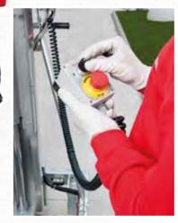
The emovable control allows the platform to be raised from the ground.
